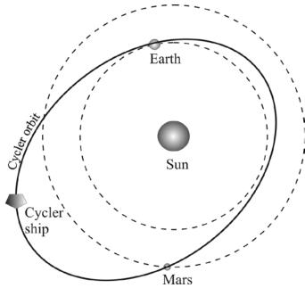
Basic idea of a cycler orbit. This orbit intercepts with both Earth and Mars orbits.
